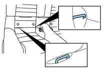
**WARNING:** The center of the rear seat is **NOT** designed as a seating position and is not equipped with safety belts. The LATCH anchors were not designed to be used with a child seat in the center position and there is no tether anchor available at the center. Attempted use of the center as a seating position will increase the risk of injury or death in the event of a collision.
